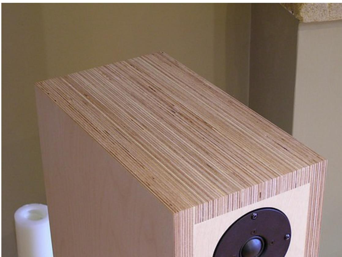
not veneered ) with the end grain of the laminated birch ply which forms the top and side panels on show making for a very neat contrast to the surface finish of the ply on all the other faces of the ply's lamination which are at right angles. It's easier to see this in the pictures than try to describe. The decision was made to leave the finish like this as veneering wasn't needed and makes for what I think is a pleasant change to the usual veneered
